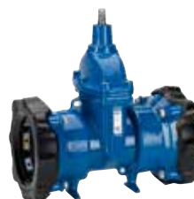
Series 636 Supa Maxi™ gate valve Universal and tensile coupling ends for all pipes DN80-300 PN16 Ductile iron
