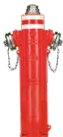
Series 84/05 Above-ground fire hydrant Break-away design with additional ball shut-off Model P7 DN80/100 PN16 Ductile iron
