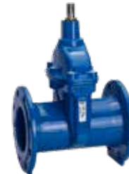
Series 02/75 Flanged gate valve Face-to-face DIN F5 Replaceable stem sealing DN40-500 PN10/16 Ductile iron
