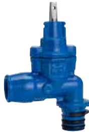
Series 103/31 Angle service connection valve with Supa Lock™ spigot/push-in socket end DN32 PN16 Ductile iron
