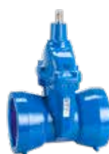
Series 33/00 Gate valve with socket ends for cast iron pipes DN80-300 PN16 Ductile iron With internal enamel
