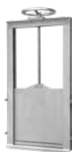
Series 772/7172 Channel penstock Uni-directional up to and incl. 1000 x 1000 mm, bi-directional in larger sizes With non-rising stem Stainless steel AISI 304 200 x 200 mm - 2000 x 2000 mm
