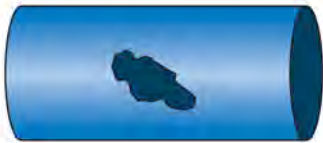
Holes in AC, steel or cast iron
