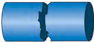
Breaks in AC and cast iron pipes
