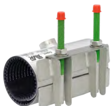
729/D2 (FST 20) Double band repair clamp, EPDM,ribs, stainless steel 304/316 with flanged outlet 10/16 bars
