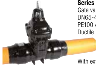
Series 36/90 Gate valve with PE ends DN65-400 PE100 / PN10 SDR 11
