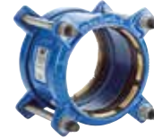
Series 621/10 Supa Plus™ coupling Tensile for PE and uPVC pipes DN32-300 PN16 Ductile iron
