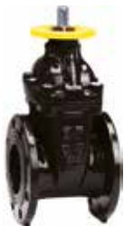
Series 15/78 Flanged gate valve with ISO top flange DN50-400 PN10/16 Ductile iron With external PUR coating
