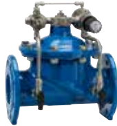
Series 859/001X Control valve Pressure sustaining DN50-300 PN10/16 Ductile iron / AISI 316
