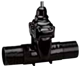
Series 46/70 Gate valve with long spigot ends DN50-600 PN16 GS-C 25 N With external PUR coating
