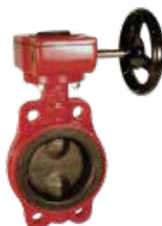
Series 75/31 Butterfly valve Centric with fixed liner Semi lug DN50-300 PN10/16 Ductile iron FM approved
