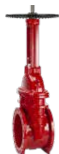
Series 55 Flanged gate valve with rising stem OS&Y DN450-600 13.7 bar (200 PSI) PN16 drilling 316 stem Ductile iron UL/ULC listed, FM approved
