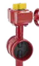
Series 815/40 Butterfly valve Centric with rubber Vulcanised disc Grooved ends to AWWA C606 DN65-200 24.1 bar (300 PSI) Ductile iron UL/ULC listed, FM approved
