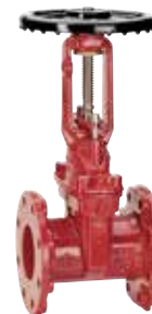
Series 145/46 Flanged gate valve with rising stem OS&Y DN50-200 17.2 bar (250 PSI) ANSI drilling class 150 Ductile iron UL/ULC listed, FM approved
