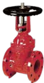
Series 45/56 Flanged gate valve with rising stem OS&Y DN50-300: 17.2 bar (250 PSI) DN350-400: 13.7 bar (200 PSI) PN16 drilling Ductile iron UL/ULC listed, FM approved
