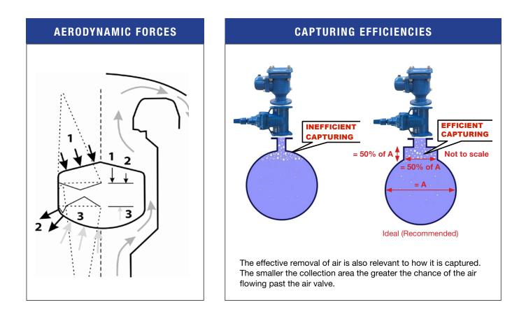
The end result is, if the valve is sized correctly and capture area is maximised, efficiencies will be improved. Below is a graph showing pump run time before and after the installation of the AVK Series 851/50 Air Release Valve.
